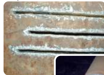
An example of cutting a rough part of SCh-20 60mm thick
