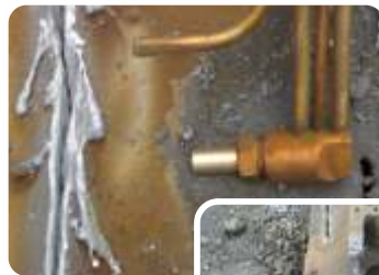
An example of cutting a sheet of metal 12x18H10T 20mm thick
